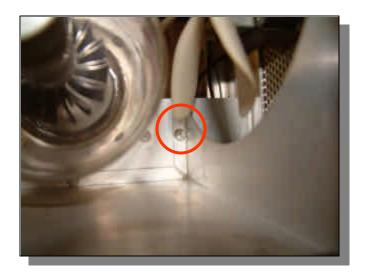
Locate the screw in the tube compartment that is held in place by this nut (it is near the corner of this compartment at the rear). Loosen this screw and remove the nut and lock washer from the underside of the chassis. Screw the threaded nylon spacer from the SK-220 kit onto the screw (freed in the previous step) and tighten well without stripping the threads in the spacer.
