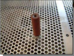
Leave this screw, it does not prevent the cover from coming off. It holds the shaft that shuts the unit down if the cover is removed while powered up. Your amp may not have this, but it should.
